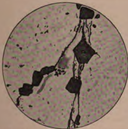
FIG. 9.—CRYSTALS OF PYRITE FORMING BY REPLACEMENT IN CHLORITIC DIABASE ALONG CRACKS FILLED WITH CALCITE. GREAT NORTHERN MINE CANYON, IDAHO \blacktriangle = PYRITE; BLACK = CALCITE; SHADED = CHLORITE. (MAGNIFIED 12 DIAMETERS. LINDGREN)
